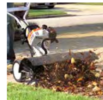
KB-MM BRISTLE BRUSH ATTACHMENT Make quick work of sweeping jobs on walkways and other paved surfaces. NOTE: This attachment must be used with large deflector and extensions. Do not use on grass lawns.
