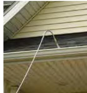
GUTTER CLEANER Gutter cleaner allows you to clean the inside of a gutter from the ground.
